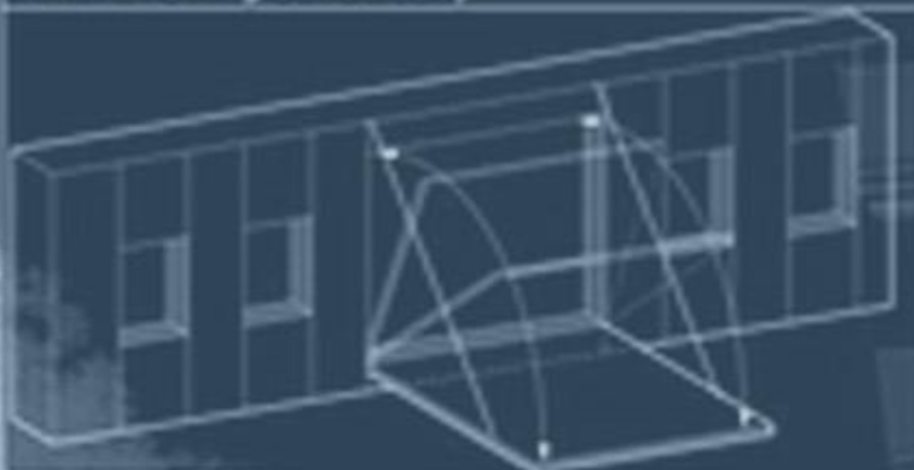
Prefabricated Facade Element with a "Swing-out Balcony"
