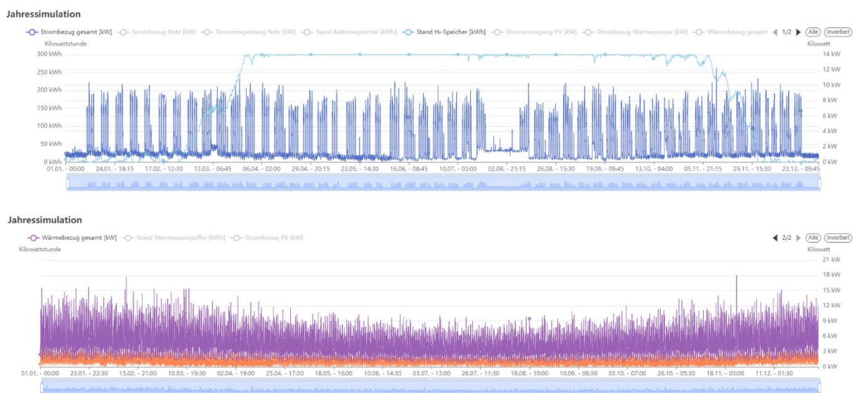
Figure 12: Results of a simulation (H2-storage, power consumption and heat delivery of a heatpump system) Johann control unit
