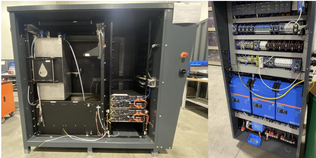
Figure 15: the new, modular and “tidied” structure of JOHANN
