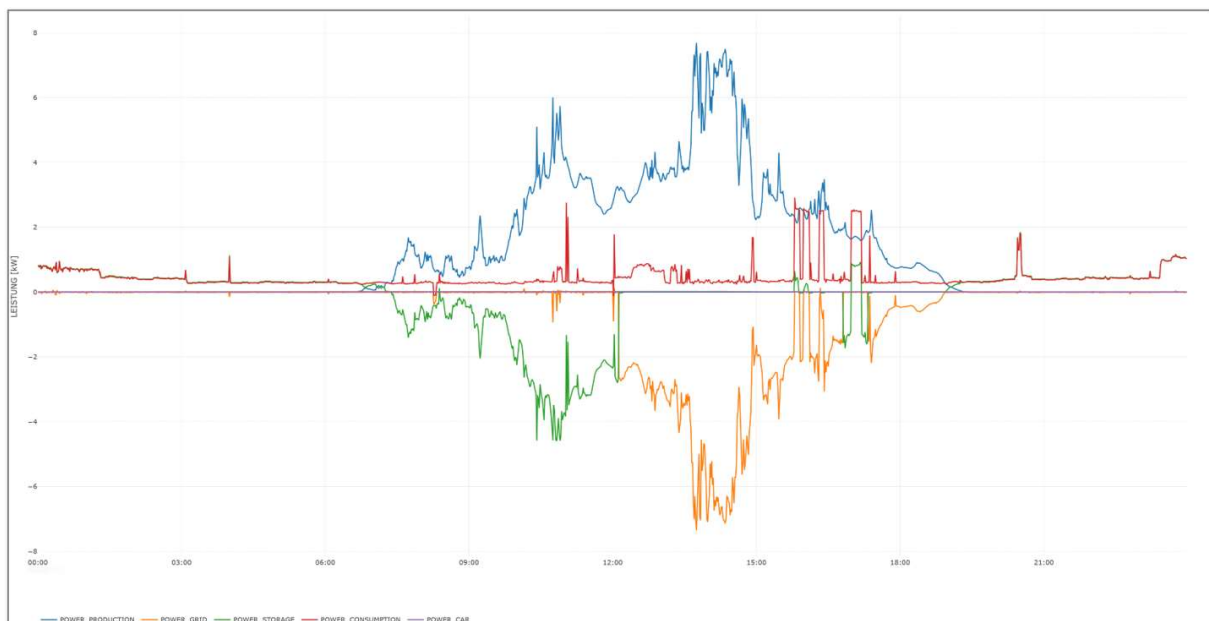
Figure 16: Historical Dashboard Data - Historical data view from the dashboard, showing past energy production, consumption, and storage performance for analysis and optimization purposes (RSO).
