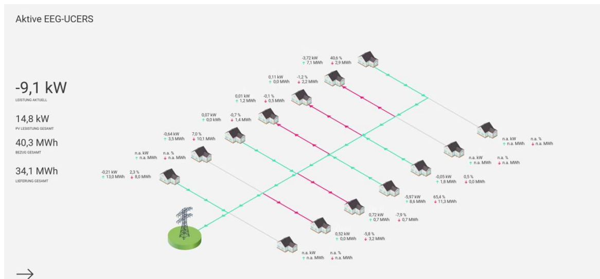
Figure 15: Dashboard: Production & Storage - Energy community dashboard for the COOP, displaying energy production, consumption, & storage activity (RSO).
