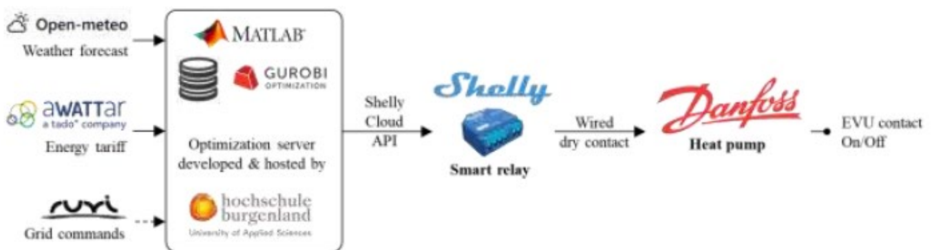
Figure 26: Automation and communication setup for the final PnP control demonstration in the PLBG building (Source: FH Burgenland, 2024)
